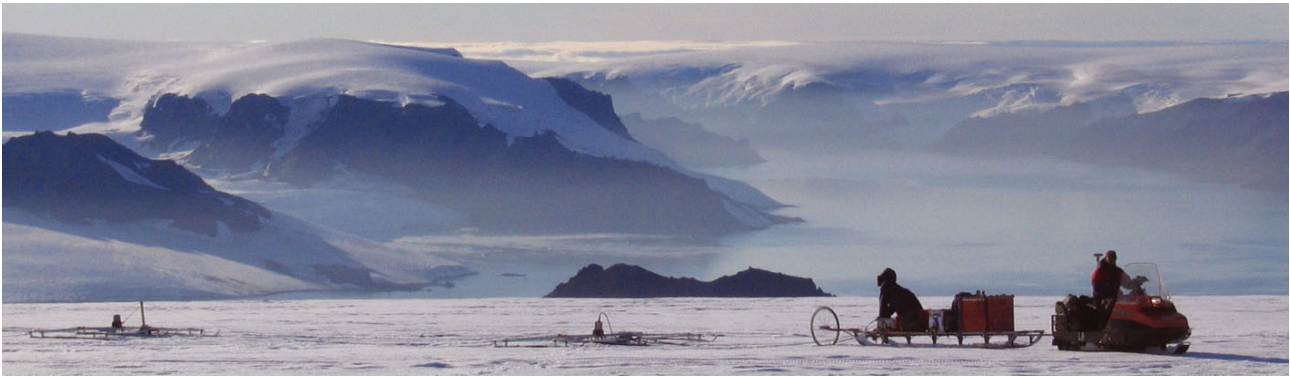
Fig. 3. The GPR antennae and a sledge with the GPR control unit are dragged by a snowmobile with a DGPS system.
