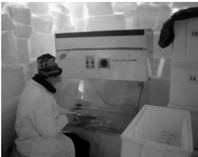
Fig. 3 – Sub-sampling the Lange IC, in a snow trench, under a portable laminar flow bench (background).
