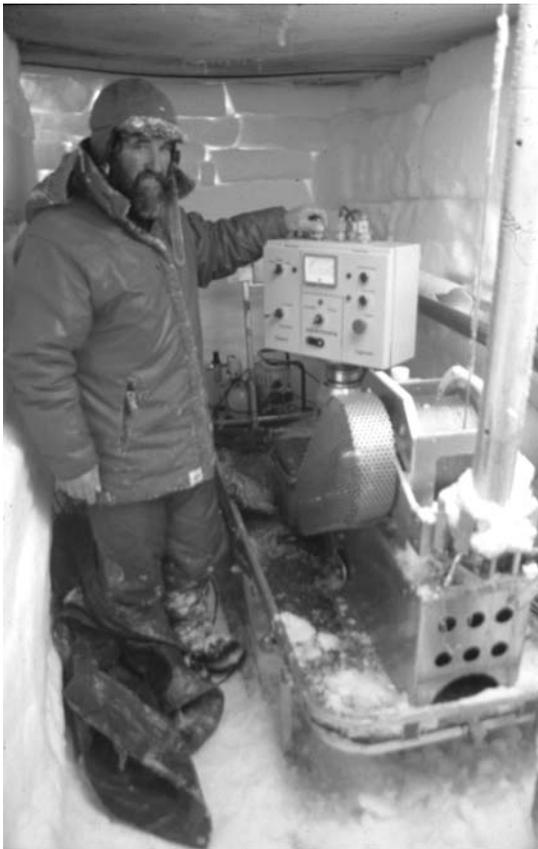
Fig. 2 – Portable electro-mechanical drill used for drilling the Lange IC (49.9 m).
