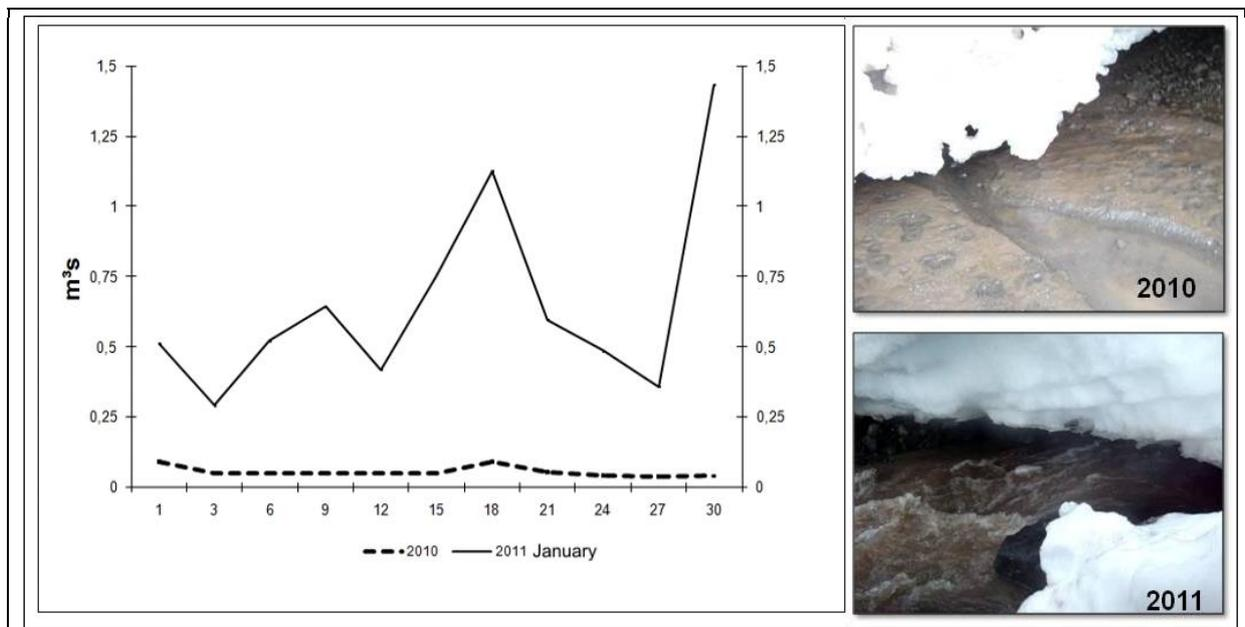
**Figure 7.** Discharge in proglacial channels when comparing January 2010 and 2011.
