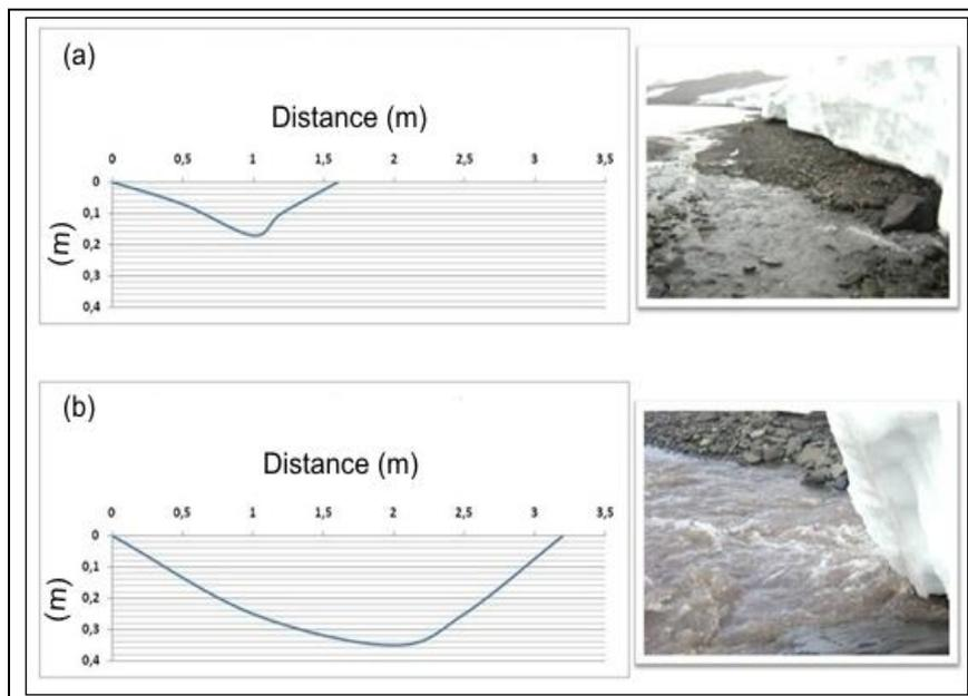
**Figure 6.** Fluctuations of the channel cross section morphology due peaks in proglacial discharge (a) obtained on January 2010 and (b) obtained on January 2011.
