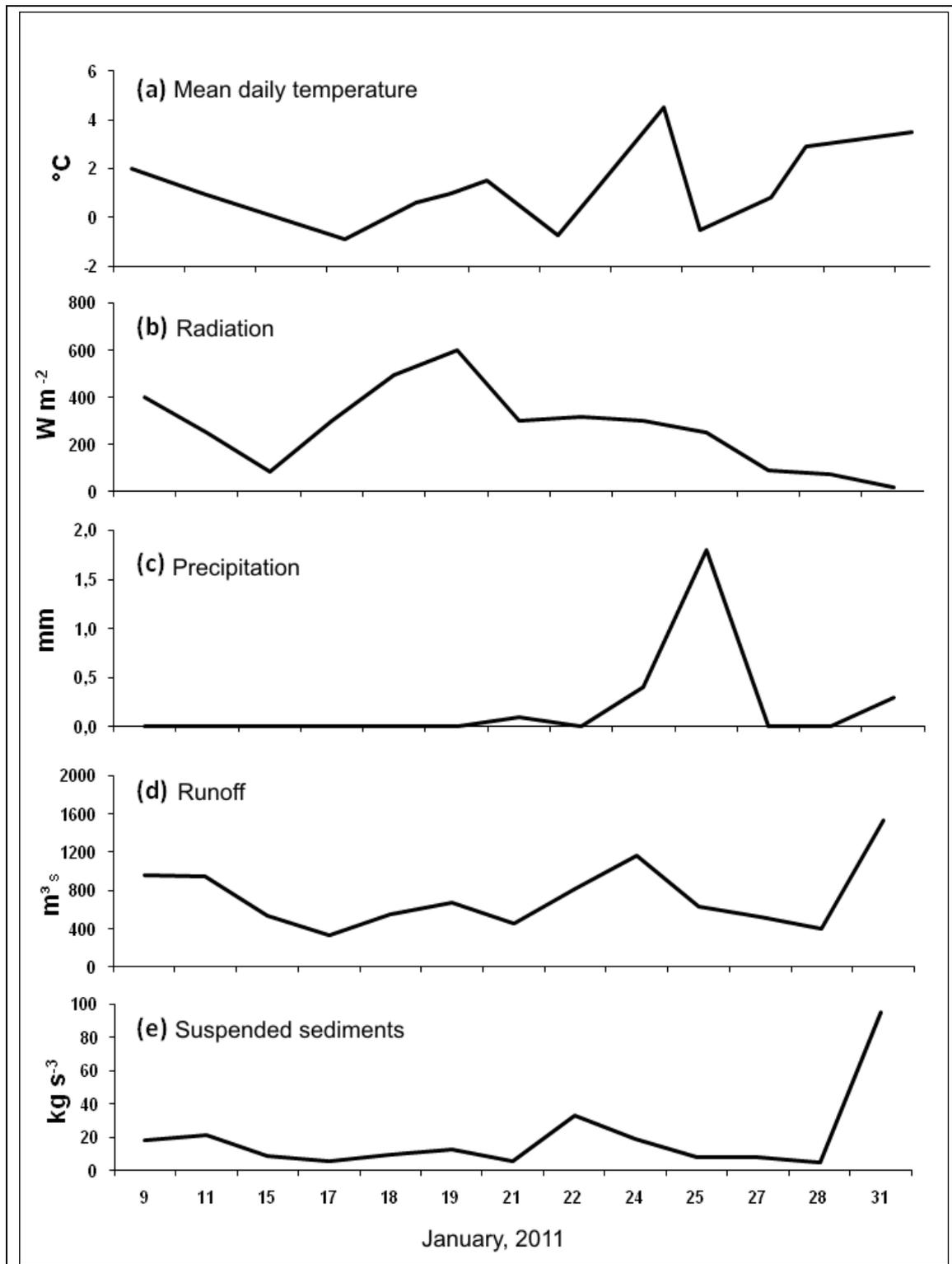
**Figure 5.** Temporal variations of air temperature (a), radiation (b) and precipitation rate (c), runoff (d) and suspended sediment loads (e) at site in January, 2011.
