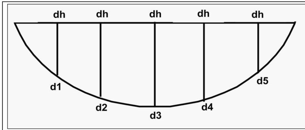
**Figure 3.** Cross sections channel measurements for partial discharge estimative. The partial discharge of each section (dh) was estimated by multiplying the water flow velocity by its influence area (A.Vm).
