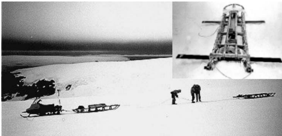
Fig. 2 – Snowmobile train for the common-offset profiles. The GPS antenna is mounted on the snowmobile. The GPR console is mounted on a Nansen sledge, next to the snowmobile, and the antennae on a second sledge some 15 m away from the first sledge. The antennae are securely tied to the bottom part of the sledge as seen in the inset. The large picture was taken on Lange Glacier, looking SE towards Admiralty Bay.
